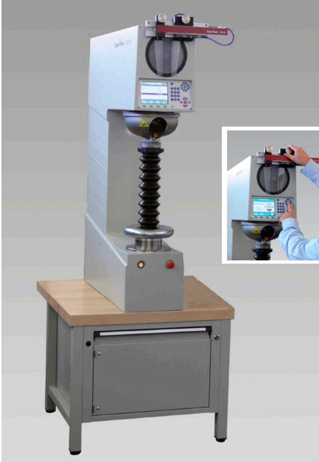
Zwick/ZHU250 Universal Hardness Tester
